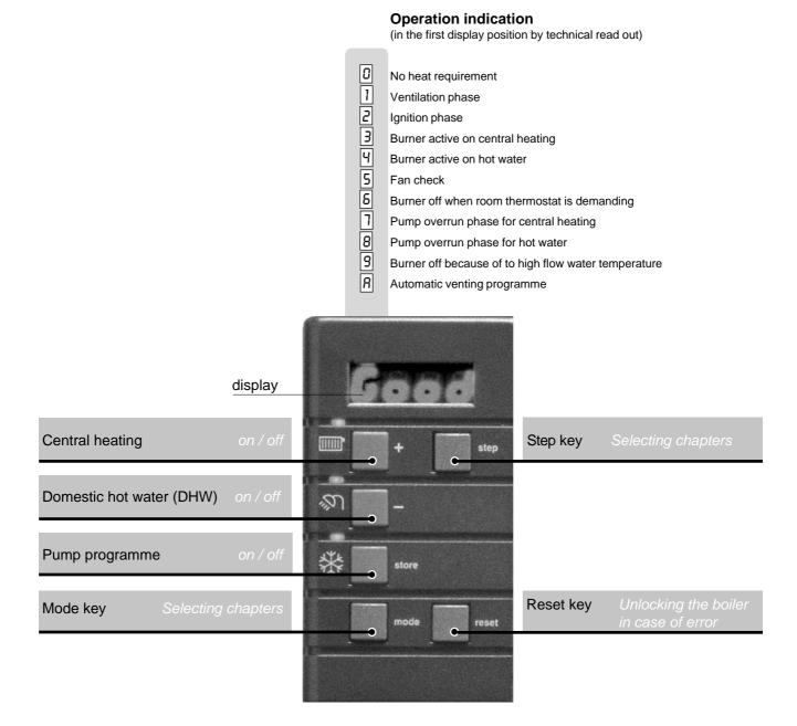
From Good-read out to Technical read out (and vice versa): - Press 5 sec. on the STEP key.
