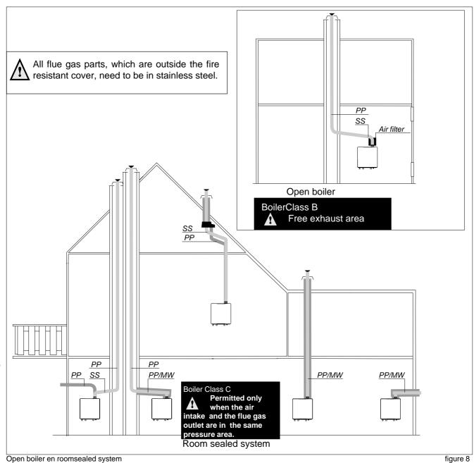
The appliance connection diameter is 80/125 mm, to which the flue gas outlet and air supply system can be fitted, with or without elbow pieces. The maximum permissible pipe length is set out in Table 5.
