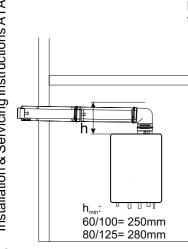
The flue diameter is determined by the total length of the run, including for the connection pipe, elbows fittings and terminal covers etc and the type and number of boilers installed into the system.
