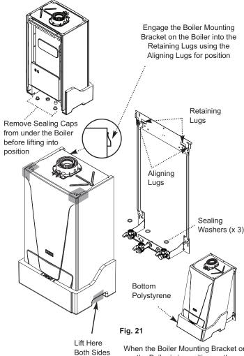
When the Boiler Mounting Bracket on the Boiler is in position on the Retaining Lugs, the bottom polystyrene may be discarded allowing the boiler to swing into position
