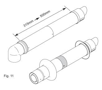
Ensure that no part of the white outer chimney duct is visible
