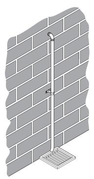
The end of the pipe should terminate facing down and towards the wall
