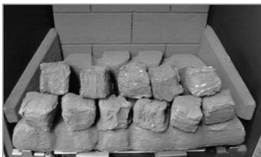
Place the rear row of four coals, making sure that the flat sides are firmly against the brick panel and side cheeks as shown.
