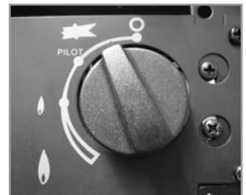
To achieve the HIGH setting, push the control knob in slightly and continue turning anti-clockwise to the high position. The main burner should light after a few seconds.
