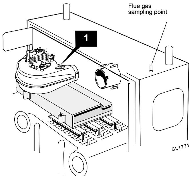
9. Remove all loose deposits from the heat exchanger, particularly between the fins, using a suitable brush.
