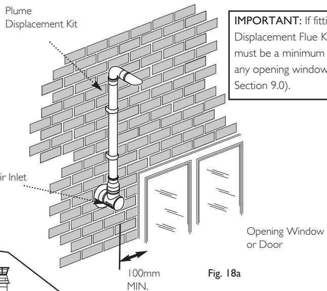
**IMPORTANT:** If fitting a Plume Displacement Flue Kit, the air inlet must be a minimum of 100mm from any opening windows or doors (see Section 9.0).
