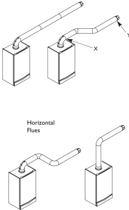
**NOTE:** Horizontal flue pipes should always be installed with at least a 1.5° fall from the terminal to allow condensate to run back to the boiler.
