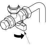
Heating Flow, Heating Return and Mains Water Inlet Isolating Valves
