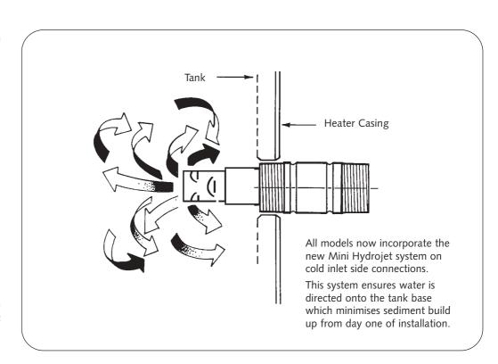
Hydrojet Inlet Nipple (Front Cold Inlet Connection)
