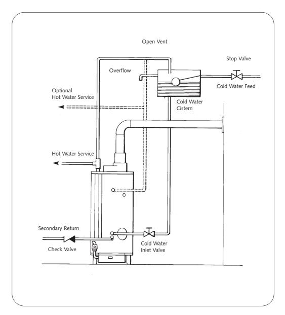
**Fig 10.** Typical Installation Vented System
