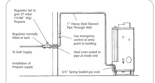
BULK STORAGE VESSEL INSTALLATION
