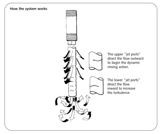
The heater is fitted with the Hydrojet Total Performance System incorporated in the cold inlet dip tube. The tube is designed to increase turbulence and reduce sediment build up, reduce thermal stacking and increase delivery.
