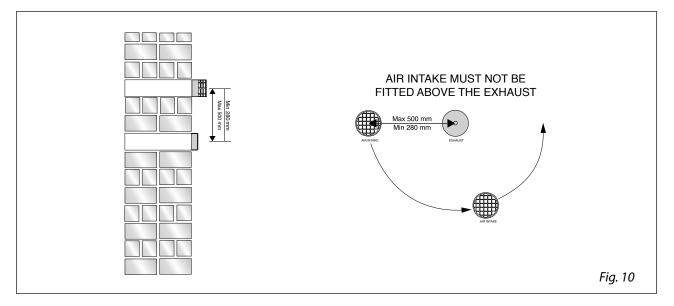
For coaxial systems, the maximum development value, mentioned in the table below also takes into account an elbow.
