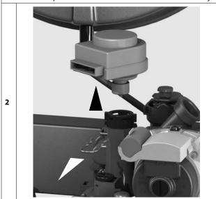
Drain the boiler (see 3.3). Remove the clip and lift the diverter valve from the assembly.
