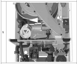
Remove the two clips and disconnect the pipes. Isolate the gas supply and disconnect the gas pipe. Remove the four screws.
