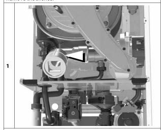
Isolate the gas supply. Disconnect the gas pipe.
