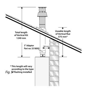
Once the boiler has been positioned on the wall, it is necessary to insert the Ø80/125 adaptor (Fig. 5) for both horizontal and vertical flue runs into the boiler flue socket (not supplied with flue kit - Part No 3318095).
