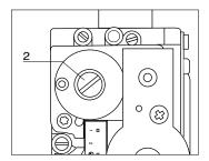
Attention! If the value of the CO2 at the minum power has been changed, it is necessary repet the adjusting at maximum gas flow.
