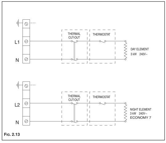
The thermostat(s) on the immersion heater(s) should be adjusted to trip at 60°C. This is the ideal temperature to prolong element life in hard water areas. Scale on the sheath builds up more rapidly at temperatures above this causing the element to overheat and premature failure can occur. Higher temperatures without additional controls would result in scalding.
