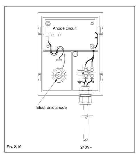
The *ProTech* system, an exclusive solution, is an electronic anti-corrosion protection system which ensures maximum longevity of the appliance, regardless of water quality. The electronic circuit creates a difference in potential between the hot water tank and the titanium electrode, thereby guaranteeing optimum protection of the tank and preventing corrosion.
