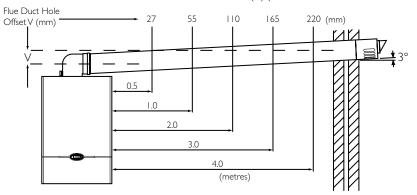
Distance in metres from boiler to the wall. For pipe lengths greater than 4m increase the off-set by 52mm for every additional metre to maintain approx 3° inclination.
