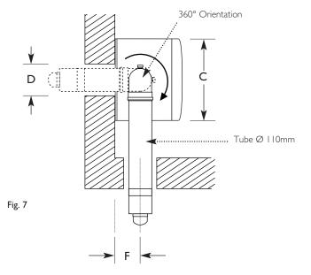
The 3° (1 in 20) fall provided by the elbow is to allow condensate to run back to the boiler, for disposal through the condensate discharge pipe.
