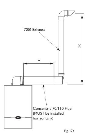
**IMPORTANT:** If fitting a Plume Displacement Flue Kit, the air inlet must be a minimum of 100mm from any opening windows or doors (see Section 7.9).
