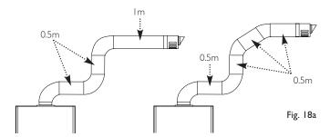
Pictorial examples of flue runs where EQUIVALENT flue length equals 4m
