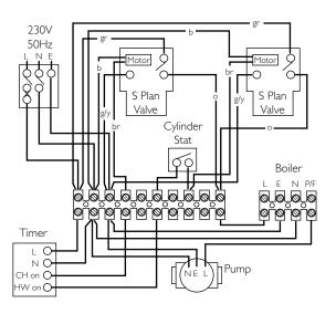
S Plan, Fully TRV'd System, CH Interlocked By Boiler Flow Switch
