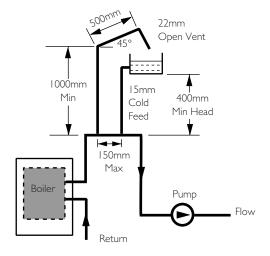
Fig. 10 Typical Low Head Installation
