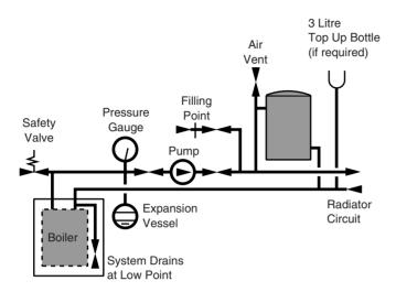
$\begin{tabular}{ll} Max \ Boiler \ Flow \\ Fig. \ 9 & Temp = 82^\circ \ C \\ \end{tabular}$
