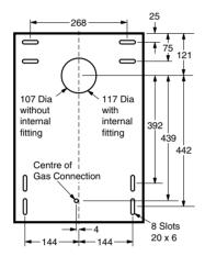
Layout of Fixing Points 30, 40 and 50 models
