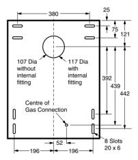
Layout of Fixing Points 60, 70 and 80 models
