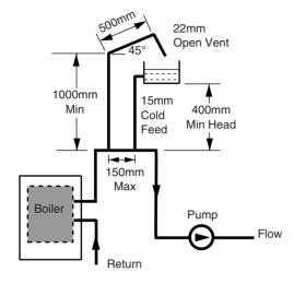
Fig. 6 Typical Low Head Installation
