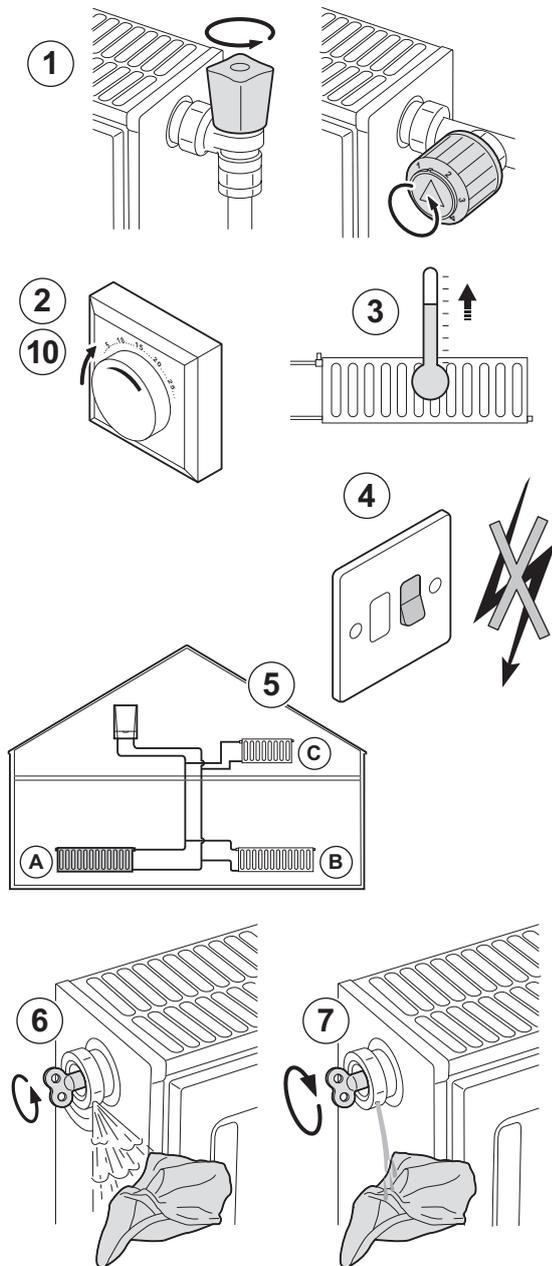
If any air is present in the appliance or system it must be removed in order to prevent nuisance noises that may occur during operation. The boiler has an inbuilt auto air vent to aid the removal of air and is supplied in the open position. Proceed as follows:
