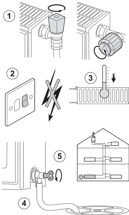
It may be necessary to drain the CH system if radiators need to be replaced or removed, if there is a major water leak or if there is a risk of freezing. Proceed as follows:
