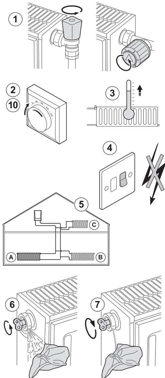
1. If any air is present in the appliance or system it must be removed in order to prevent nuisance noises that may occur during heating or when drawing off hot water. Proceed as follows:
