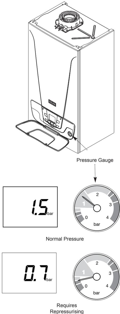
1. If the water pressure is too low, the installation must be re-pressurised.
