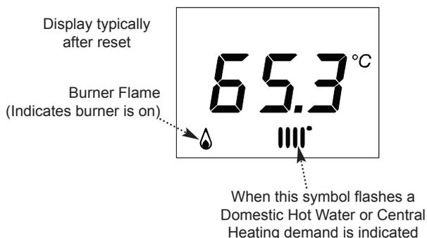
1. In the unlikely event of an error occurring the display will show one of two symbols or **R**. In both cases the display will also show **E** symbol and the numeric value of the error (see the 'Table of Error Codes').
