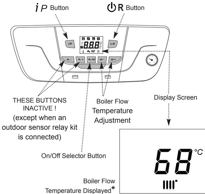
The values displayed are the temperature as measured at the boiler, not necessarily that at the radiator or tap. Because of differences in systems, seasonal variations in mains water temperature etc. some adjustment of the temperatures may be required to achieve the desired results. Your installer will be able to offer advice.
