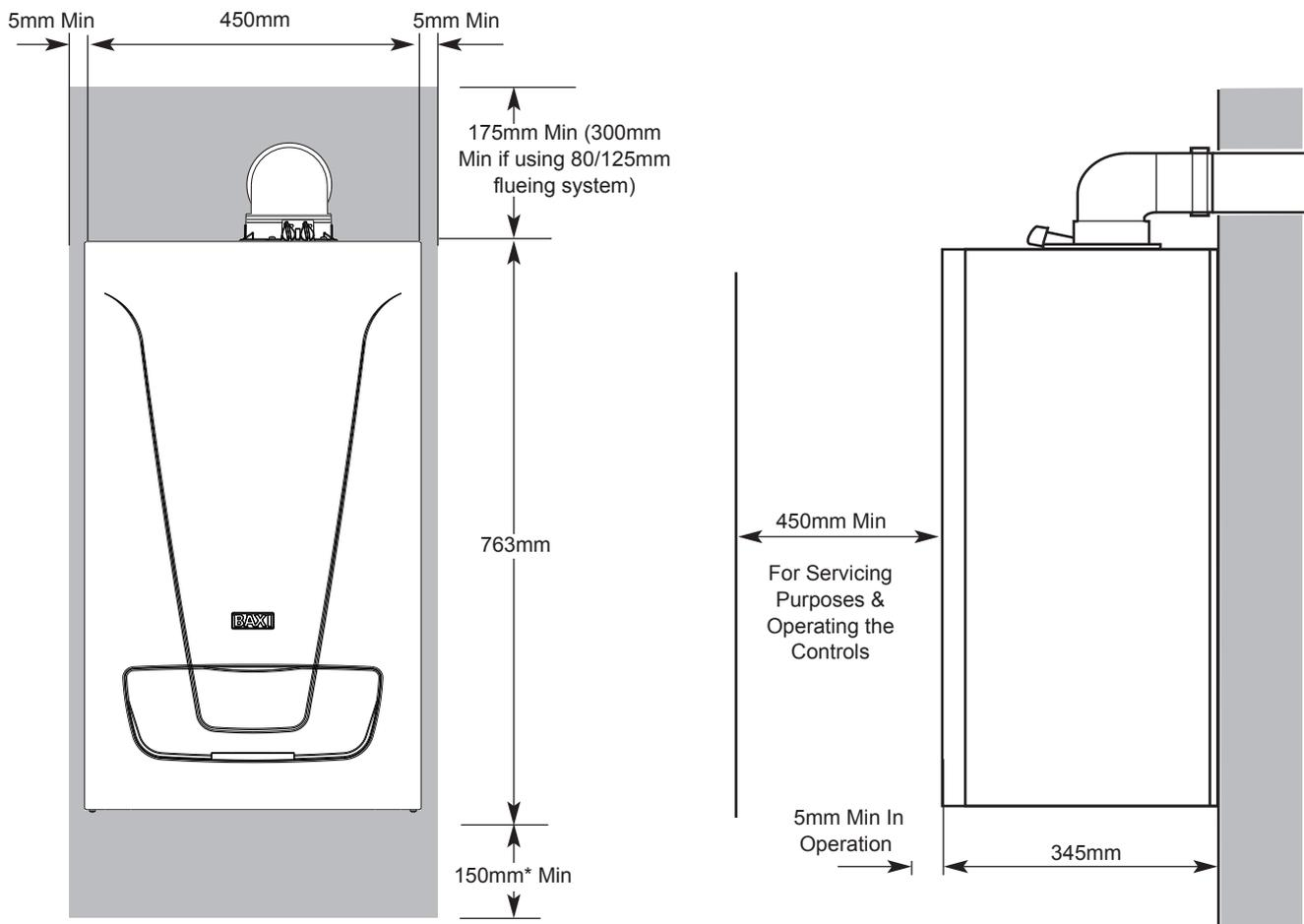
\*This is MINIMUM recommended dimension. Greater clearance will aid installation and maintenance.
