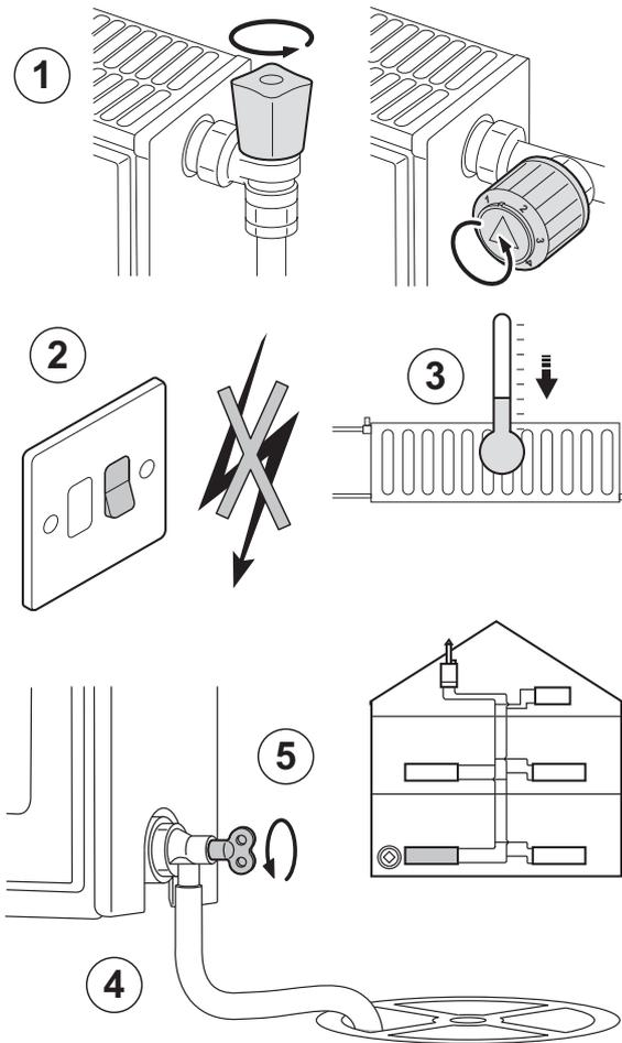
1. It may be necessary to drain the CH system if radiators need to be replaced or removed, if there is a major water leak or if there is a risk of freezing. Proceed as follows:
