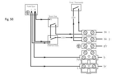
NOTE: The 230V switched signal for external controls (Frost Stat - Room Stat - Timer) must always be taken from terminal 2 at the boiler. Live, Neutral and Earth to power these controls must be taken from the Fused Spur.
