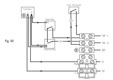
NOTE: The 230V switched signal for external controls (Frost Stat - Room Stat - Timer) must always be taken from terminal 2 at the boiler. Live, Neutral and Earth to power these controls must be taken from the Fused Spur.
