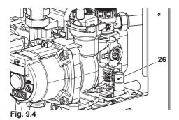
A small quantity of water will remain in the d.h.w. heat exchanger after draining. If the boiler is being drained to prevent freezing, the d.h.w. heat exchanger must be removed and inverted to drain fully or an antifreeze solution added.
