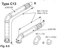
Co-axial 60/100 mm - nominal length 1 m This kit can be fitted to allow discharge to the rear or either side of the boiler via the flanged boiler adapter elbow. Minimum length required is 0.3 m. Maximum equivalent length of 10 metres can be achieved utilising extensions. This flue system can only be used to discharge horizontally, it is not designed to enable termination in the vertical plane.
