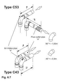
N.B: The air intake and the flue outlet must not terminate on opposite sides of the building.
