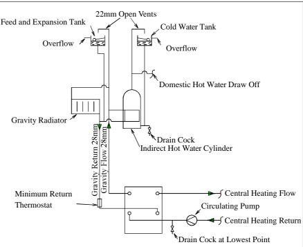
Fig. 5. Typical Central Heating & Hot Water System
