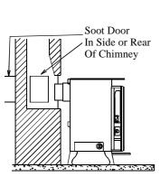
Fig 8. Vertical Register Plate With Bricked Up Fireplace
