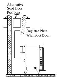
Fig 9. Horizontal Register Plate With Rear Flue Connection
