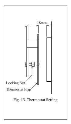
re-tighten the locking nut. Ensure that the flap opens and closes freely as the knob is turned.
