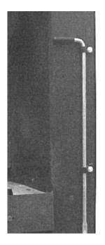
Flip the slide control lever round so that the rubber-capped end is protruding out to the right as shown in the left-hand picture. Check that it slides freely up and down in the nylon slide guides. Remove the nyloc nut with a 7mm A/F spanner as shown
