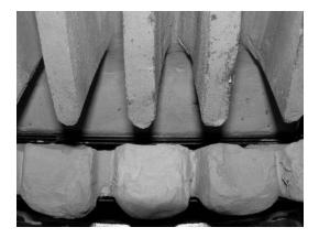
• slide front coal support on to the edge of the burner carrier this will support the front coal matrix and help stabilize the fuel bed
