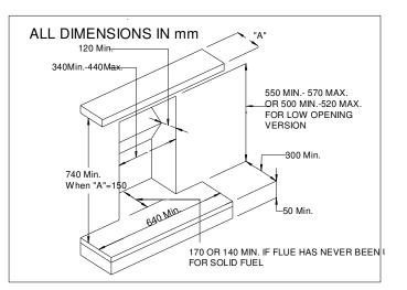
Any permanent flue restriction or variable dampers shall be removed or locked fully open. The chimney should be swept prior to installation if not new or previously used with a gas appliance.
