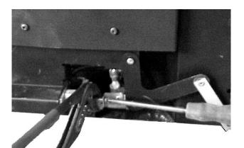
Taking great care grip the copper protective sleeve at the end of the gas control spindle (DO NOT GRIP SPINDLE IN AND OTHER PLACE) as shown and remove the screw from the end as shown above.
