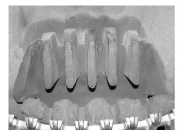
• Locate the front coal matrix with the shapes upwards in front of the rear matrix. Ensure that it is not placed on top of the burner slot.
