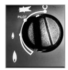
When the pilot lights after the spark, keep the knob depressed for approximately ten seconds. Now release the knob and the pilot should stay alight. If the pilot extinguishes during use, wait three minutes before repeating the ignition procedure. To achieve the HIGH setting, push the control knob in slightly and continue turning anticlockwise to the high position. The main burner should light after a few seconds. To decrease the setting to LOW, turn the control knob clockwise to the low setting.
