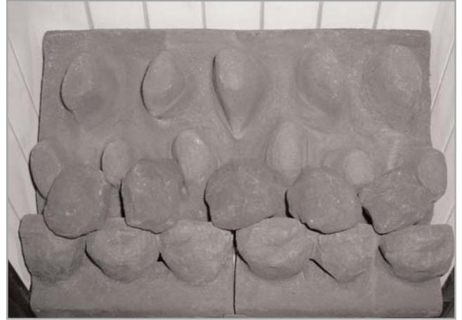
4. Take five more moulded coals and position as shown to form the 'second row' of the fuel effect. The coals may be rotated as desired to fit into the gaps between the coal supports in order to create a random, realistic effect. Again, remember not to push the coals down too far into the valleys between the coal supports as this can have a detrimental effect to the flame picture.
