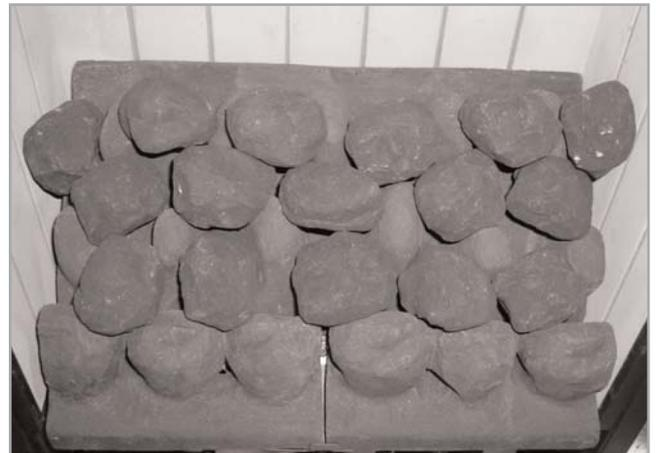
6. Finally, take the six remaining coals and place at the back of the fuel matrix, as shown. Adding these coals should complete the appearance of the fuel bed giving an even distribution of equally spaced coals.
