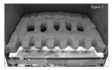
2. Place the matrix into position as shown in figure 3. Slide it back to the rearmost position and centralise.
