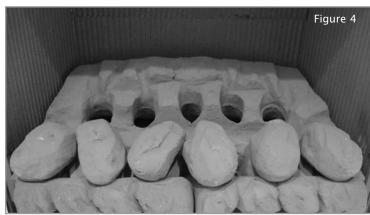
4. Open the bag of 16 moulded coals. All of the coals are the same. Take six coals and place them as shown in figure 4. Care should be taken to ensure that the coals bridge the gap between the front coal and the four coal supports at the front of the matrix.
