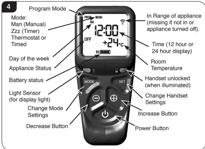
The icon at the bottom of the screen displays the battery condition of both the batteries in the handset and in the Control Box alternatively.
