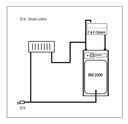
If heating of a single bathroom radiator or towel rail is required in summer, then it can be piped as a gravity circuit. The flow pipe to the radiator can be teed into the safety open vent pipe and the return pipe from the radiator can be connected to the store drain connection and the drain moved to the return pipe. The radiator can be fitted with a T.R.V. if required as long as this is suitable for gravity circulation i.e. low resistance type.
