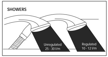
Vast quantities of water are needlessly run off to waste due to Taps, Mixers and Showers discharging flow rates far in excess of the rates required for them to perform their duties.
