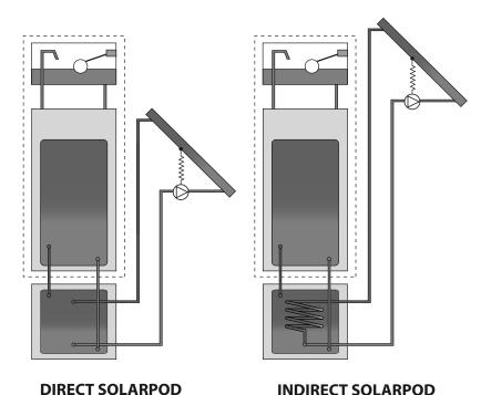
\* For indirect SolarPod, the feed cistern can be sited on top of the appliance within a minimum cupboard size of 2340mm. This still allows the minimum service height of 350mm above the cistern to service a ballvalve if necessary. Check the ceiling height is sufficient for all larger SolarPod/thermal store combinations, or arrange to relocate the feed cistern at a higher level.
