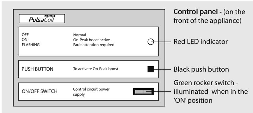
This is designed for operation by the householder and the operation is in line with the instructions on the panel.
