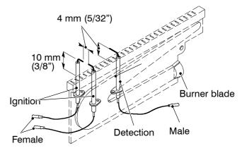
10 Check that the spark and detection electrodes leads are in good condition and renew as necessary.
