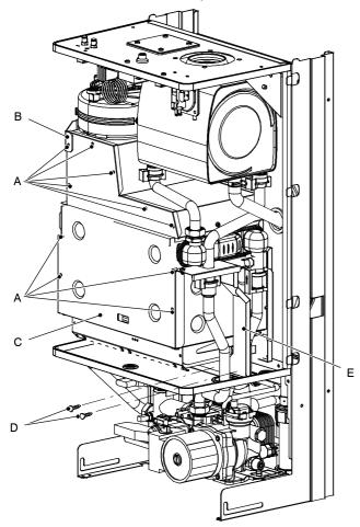
Disconnect the electrodes leads.
