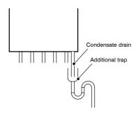
The length of the condensate pipe should be kept at minimum and must be arranged so that obstruction (e.g.
