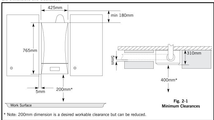
It is recommended that where the appliance is located in a kitchen, or next to other combustible materials, a gap of 5mm be left on either side and where the flue run is through a void in kitchen units, again a minimum gap of 5mm should be left.
