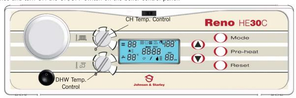
The LCD display will become active, whilst the microprocessor control completes a number of checks and sets the appliance to a standby position. When the boiler reaches its temp. set point, the anti-cycle feature introduces a 180 second delay between cycles, indicated by an hour glass symbol on the display. The display will indicate the system pressure in the lower RH corner of the LCD panel and a numerical display in the upper and lower LH side of the LCD panel.
