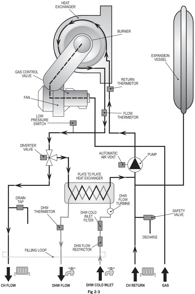
Fig 2-3 Schematic Diagram (Waterflow)
