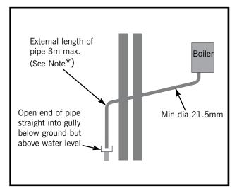
NB the boiler has a built in condense trap and it MUST be noted that fitting an additional trap to the configurations shown above, may have an edverse effect on the evacuation of condensate from the boiler.
