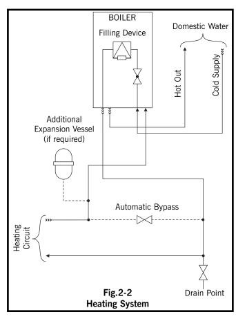
**Expansion Vessel:** The integral expansion vessel is precharged to a pressure of between 0.5 and 1.0 bar. This should be checked before the water system is filled. Details below show the water system volume that is acceptable for this vessel. If the system water volume is larger then an additional vessel must be fitted to the system. BS 5449 and BS 6798 give further details regarding expansion vessel sizing and sealed systems. See table 3-2.
