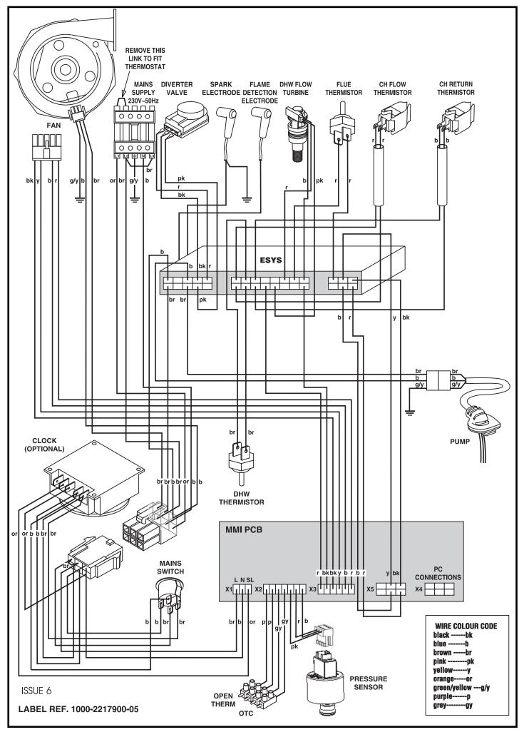
Fig.3-20 Illustrated Wiring Diagram
