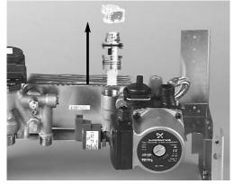
grommet. Unclip the plastic electronic component from the top of the turbine, the wires may be unplugged if necessary. Remove the grommet from the sealed chamber above the turbine. Unscrew the complete turbine from the brass housing and remove it upwards through the hole in the sealed chamber. Replace in reverse order ensuring the grommet is correctly seated.
