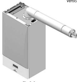
Fig.3-9 Horizontal Side Flue (Can be left or right)
