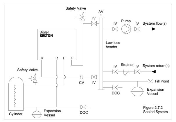
All components of the system including the heat exchanger of the indirect cylinder must be suitable for a working pressure of 3 bar and a temperature of 110 °C. Care should be taken in making all connections that the risk of leakage is minimised.
