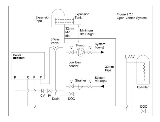
Although suitable for open vented systems with combined feed and vent arrangements, the C90 and C110 are low water content boilers. As such, any air entrainment within the system water will produce boiler "kettling". It is therefore recommended, if in any doubt, to consider the use of sealed systems where possible.
