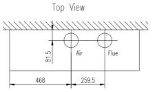
Service Connection Locations All dimensions are in mm Compartment installation is permitted. Such compartments must be constructed in accordance with BS6798.
