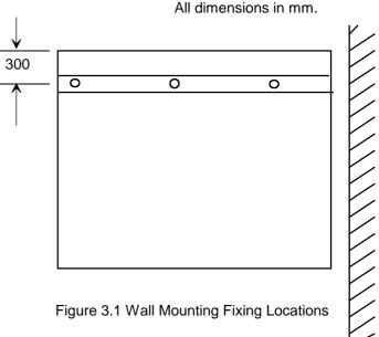
Figure 3.1 Wall Mounting Fixing Locations
