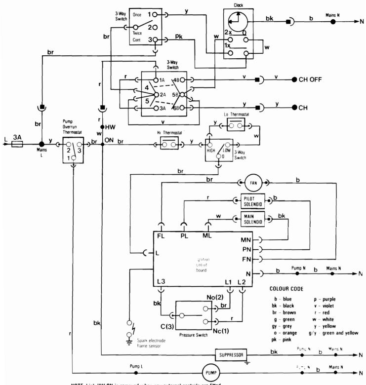
NOTE: Link HW-ON is removed when any external controls are fitted.
