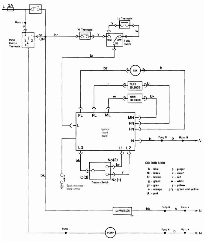
NOTE If a programmer is not fitted, link HW to ON to be removed and a switched live connected to terminal ON-
