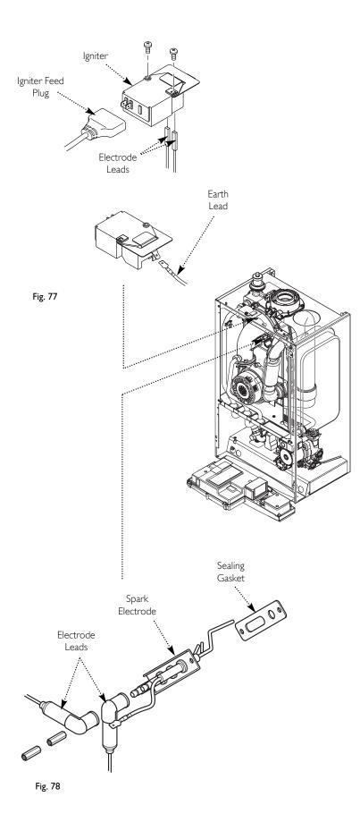
**IMPORTANT:** When changing components ensure that both the gas and electrical supplies to the boiler are isolated before any work is started. When the component has been changed turn the selector switch fully anticlockwise against the spring pressure to the reset position and hold for 5 seconds to reset the boiler before recommissioning.
