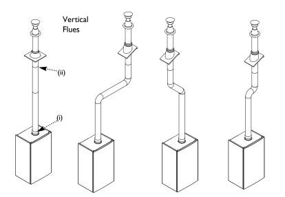
**IMPORTANT:** All flue systems must be securely supported at least once every metre. Suitable pipe supports are available as accessories.
