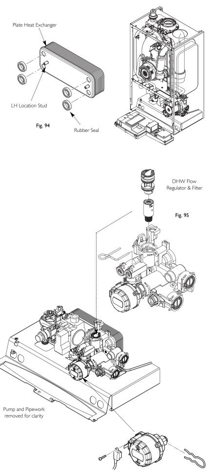
Diverter Valve Motor
