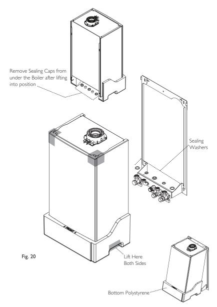
When the Boiler Mounting Bracket on the Boiler is in position on the Retaining Lugs, the bottom polystyrene may be discarded allowing the boiler to swing into position
