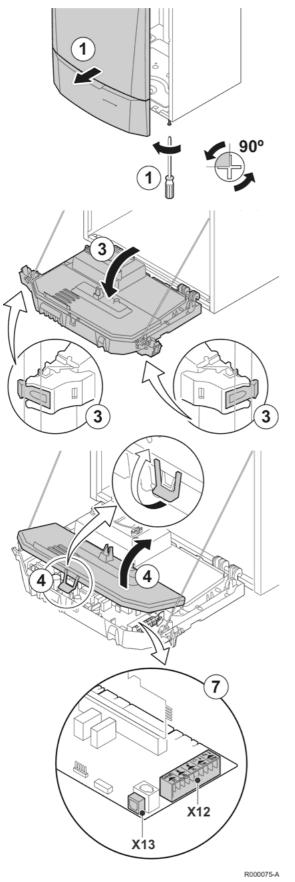
The pump must be connected to standard control PCB (PCU). To do this, proceed as follows:
