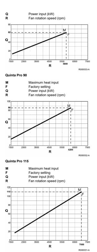
See the graphs for the relationship between heat input and speed for natural gas. The speed can be changed using parameter **P17**. To do this, proceed as follows:
