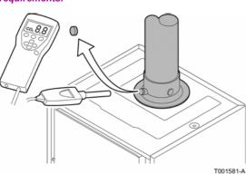
The flue gas analyser must meet the requirements of BS 7927 or BS-EN 503793 and be calibrated according to the manufacturer's requirements.
