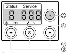
The display comprises four elements of 7 segments each. Four keys serve to make adjustments at the different operating levels.
