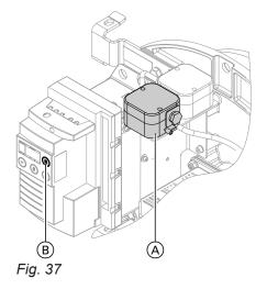
The switching threshold of air pressure switch 1 (LDW1) is monitored in all fan ramp-up phases and checked in modulating burner operation. This ensures a minimum pre-purge.
