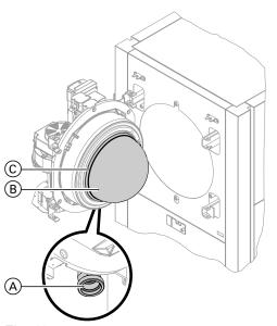
2. Undo the screws on the boiler door and open the door.
