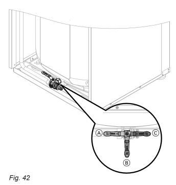
2. Connect the hose to the drain valve and route it into a suitable container or drain outlet.
