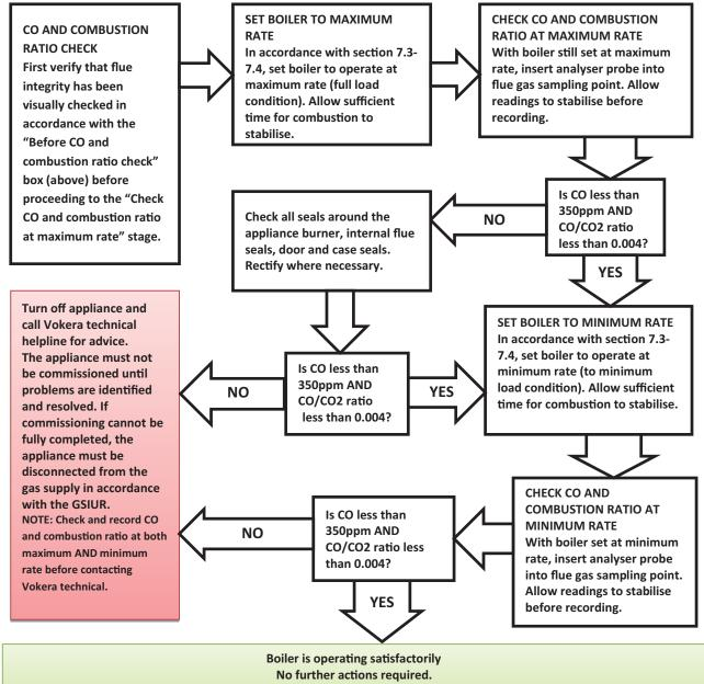
Ensure test points are capped, boiler case is correctly replaced and all other commissioning procedures are completed. Complete Benchmark Checklist, recording CO and combustion ratio readings as required.
