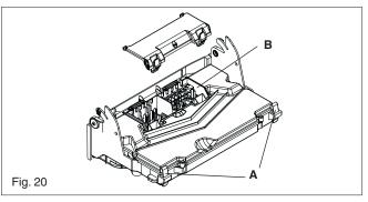
Ensure that the correct jumper tag configuration has been respected. It will be necessary to check the functioning of the PCB is set for the correct boiler type/application.
