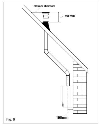
gaskets, & screws (supplied), ensuring the correct seal is made. The flue support bracket (supplied with the vertical flue kit) can now be fitted.
