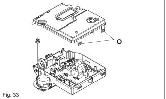
ing note of all wiring connections and jumper tag configuration. Unhook and remove connection block (P). Disconnect all wiring from the PCB, locate and remove the PCB securing screws, remove the required PCB. Replace in the reverse order ensuring that the position of the 2 control knobs are correctly aligned with the respective potentiometers on the PCB.
