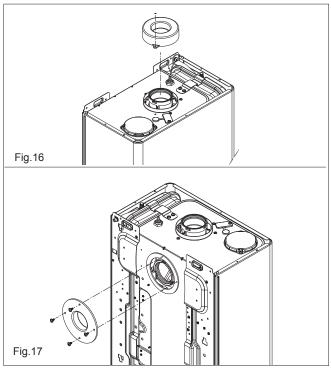
Using the screws and washers provided, secure the appliance onto the wall bracket and tighten with a suitable spanner. Seal the flue assembly to the wall using cement or a suitable alternative that will provide satisfactory weatherproofing. The exterior wall trim can now be fitted.
