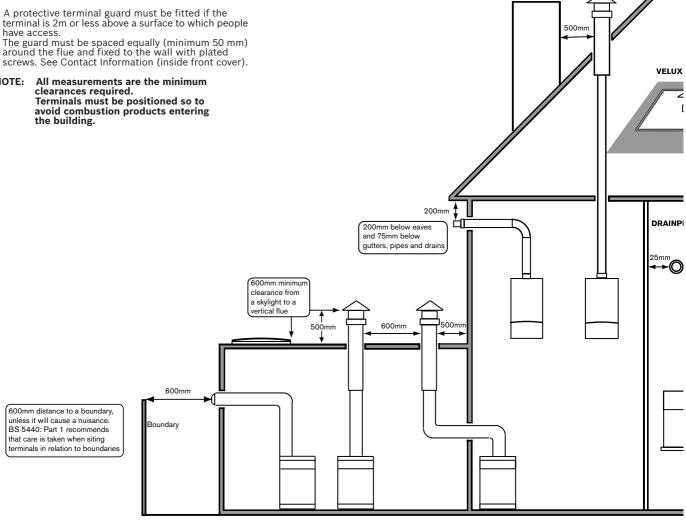
Deduct one metre off the total flue length for every 45° bend used Deduct two metres off the total flue length for every 90° bend used
