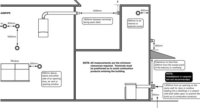
Flue clearances must be at least 300mm from the ground. Terminal guards must be fitted if the flue is less than 2 metres from the ground or if a person could come into contact with the flue terminal.
